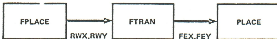
Figure 4. Flow of Control From Fisheye Routine FPLACE to Standard Graphics Routine PLACE
