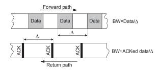
Fig. 37. Rationale for the available bandwidth estimation technique
