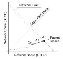
Fig. 43. Convergence diagram of the two STCP flow competition  $x_0 - x_1$ ,  $x_2 - x_1$  multiplicative increase (a flow with the larger congestion window increases more than a flow with the smaller)  $x_1 - x_2$  multiplicative decrease (a flow with the larger congestion window decreases more than a flow with the smaller)
