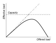
Fig. 3. Effective TCP load versus offered load from TCP senders
