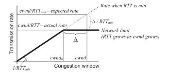
Fig. 23. TCP Vegas—the utilized buffer size  $\Delta$  as function of expected and actual rate
