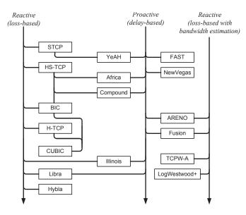
Fig. 39. Evolutionary graph of TCP variants aimed at improving efficiency in high-speed or long-delay networks
