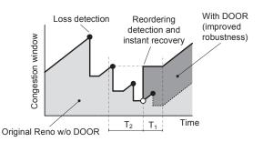
Fig. 31. Comparison of congestion window dynamics between Reno (or SACK) and DOOR
