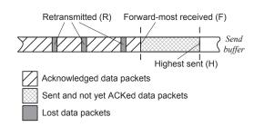
Fig. 22. Special state variables in the FACK algorithm
