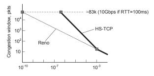
Fig. 40. Objective of HS-TCP
