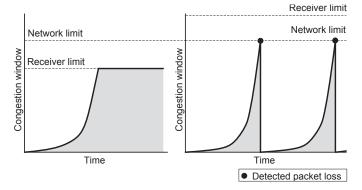
Fig. 7. Congestion window dynamics and effectiveness of *Slow-Start* if limit is imposed by legacy flow control (left) and network (right)
