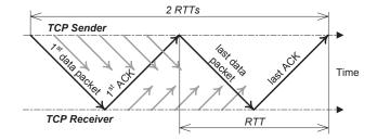
Fig. 20. The interval between the first and last data packets sent before reception of any ACK is  $2 \times RTT$  in the worst case
