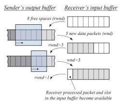
Fig. 2. Receiver's window concept: receiver reports a size of the available input buffer (receiver's window, rwnd) and sender sends a portion (window, wnd) of data packets that does not exceed rwnd
