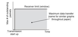
Fig. 6. Outstanding data packets allowance dynamics as defined in RFC793 (network limits are not considered)
