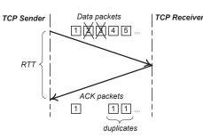
Fig. 19. Duplicate ACKs allow loss detection no sooner than after one RTT
