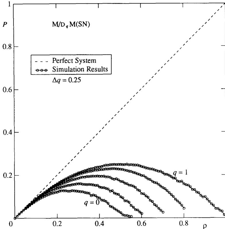
Fig. 3. Simulation results for the power in  $M/D_qM(SN)$ .
