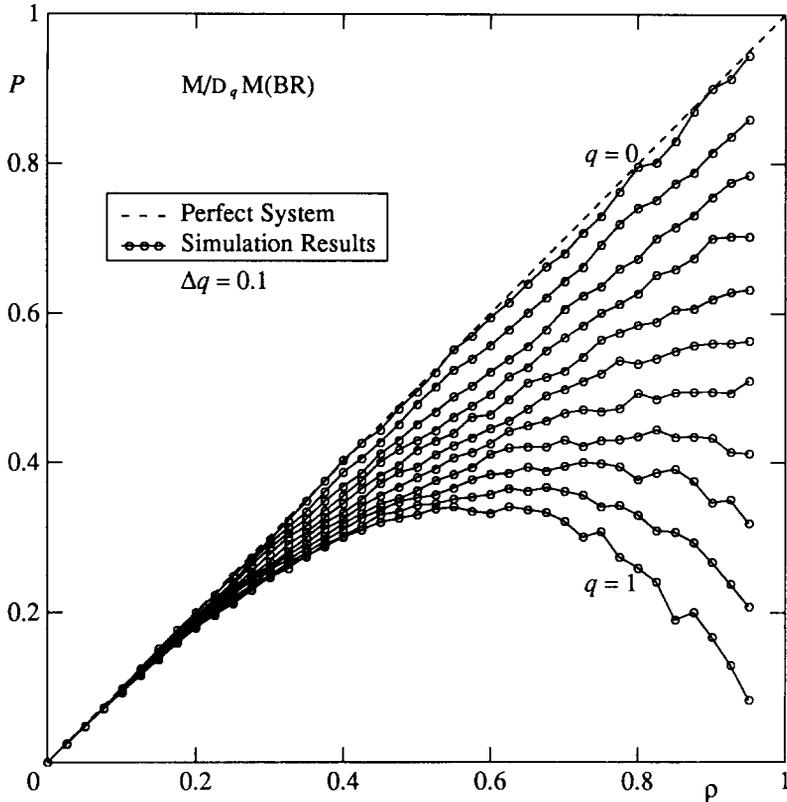
Fig. 4. Simulation results for the power in  $M/D_q M(BR)$ .
