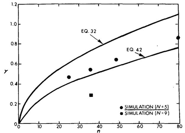
Fig. 7. Throughput for two-dimensional regular networks.
