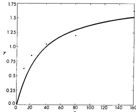
Fig. 6. Transmission probability based on an estimate of hitting degree.
