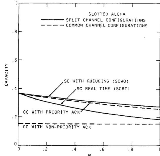
Figure 12. Slotted ALOHA: Capacity versus  $\omega$  for common and split channel configurations.
