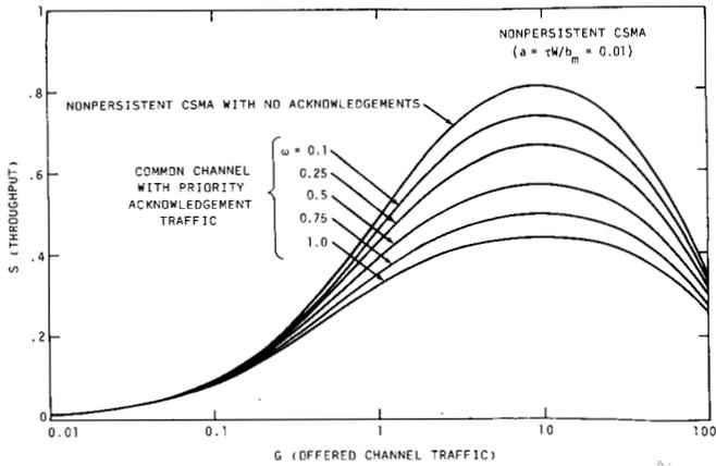
Figure 5. Nonpersistent CSMA: Throughput versus offered channel traffic.
