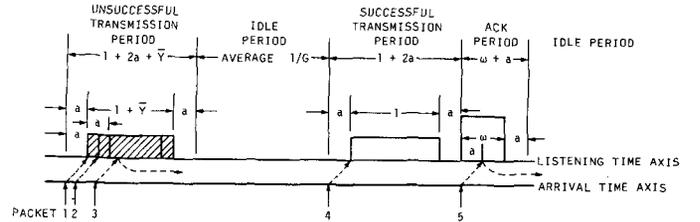
Figure 4. Nonpersistent CSMA: Common channel configuration with priority acknowledgment traffic.
