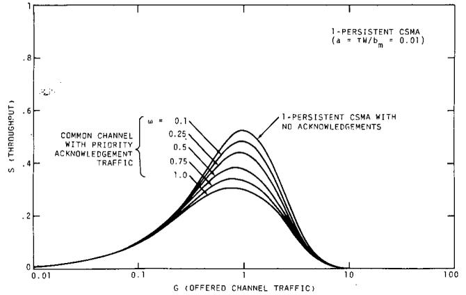
Figure 10. 1-Persistent CSMA: Throughput versus offered channel traffic.
