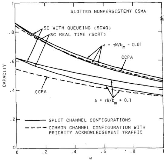
Figure 13. Nonpersistent CSMA: Capacity versus  $\omega$  for common and split channel configurations.
