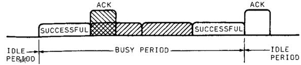
Figure 1. Slotted ALOHA: Common channel configuration with non-priority acknowledgment traffic.
