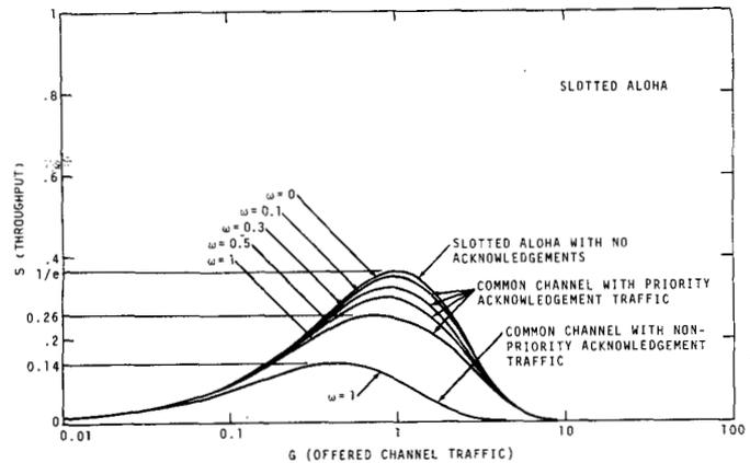
Figure 3. Slotted ALOHA: Throughput versus channel traffic.
