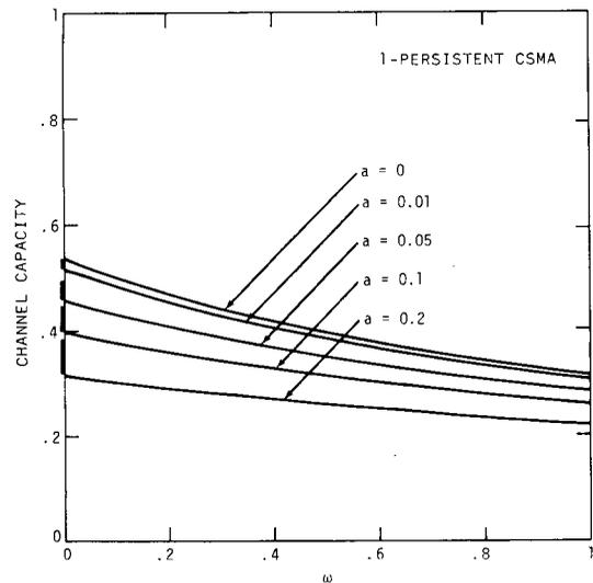
Figure 11. 1-Persistent CSMA: Capacity versus  $\omega$  in common channel configuration.
