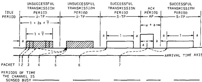
Figure 7. 1-Persistent CSMA: Common channel configuration with priority acknowledgment traffic.
