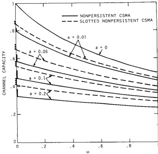
Figure 6. Nonpersistent CSMA: Capacity versus  $\omega$  in common channel configuration.
